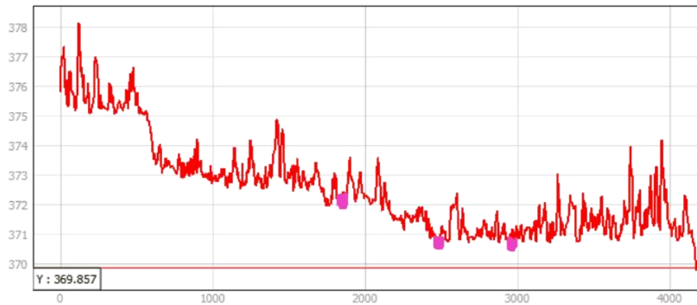
Figure 3. Proposed weir locations on longitudinal profile of the Peel River
