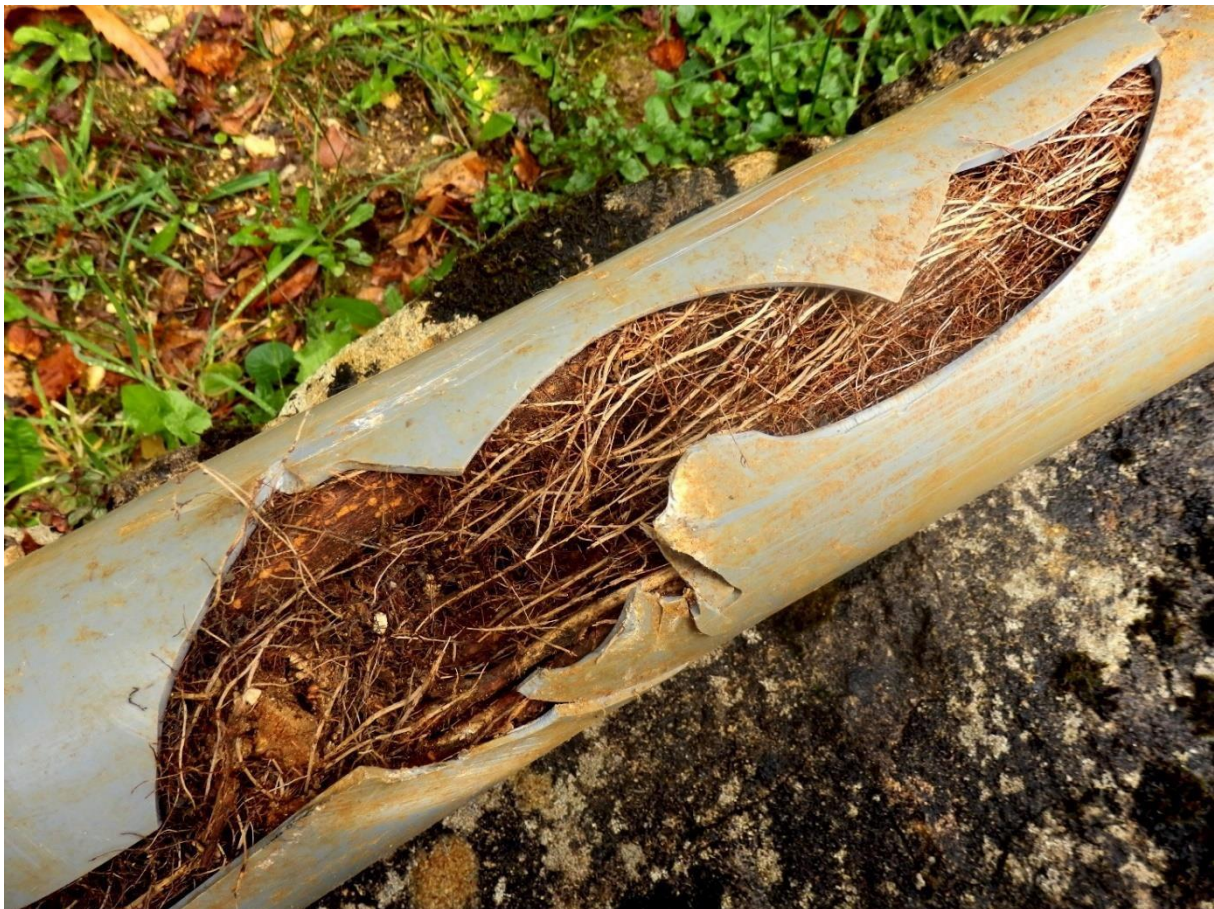
Tree root damaging stormwater drain
