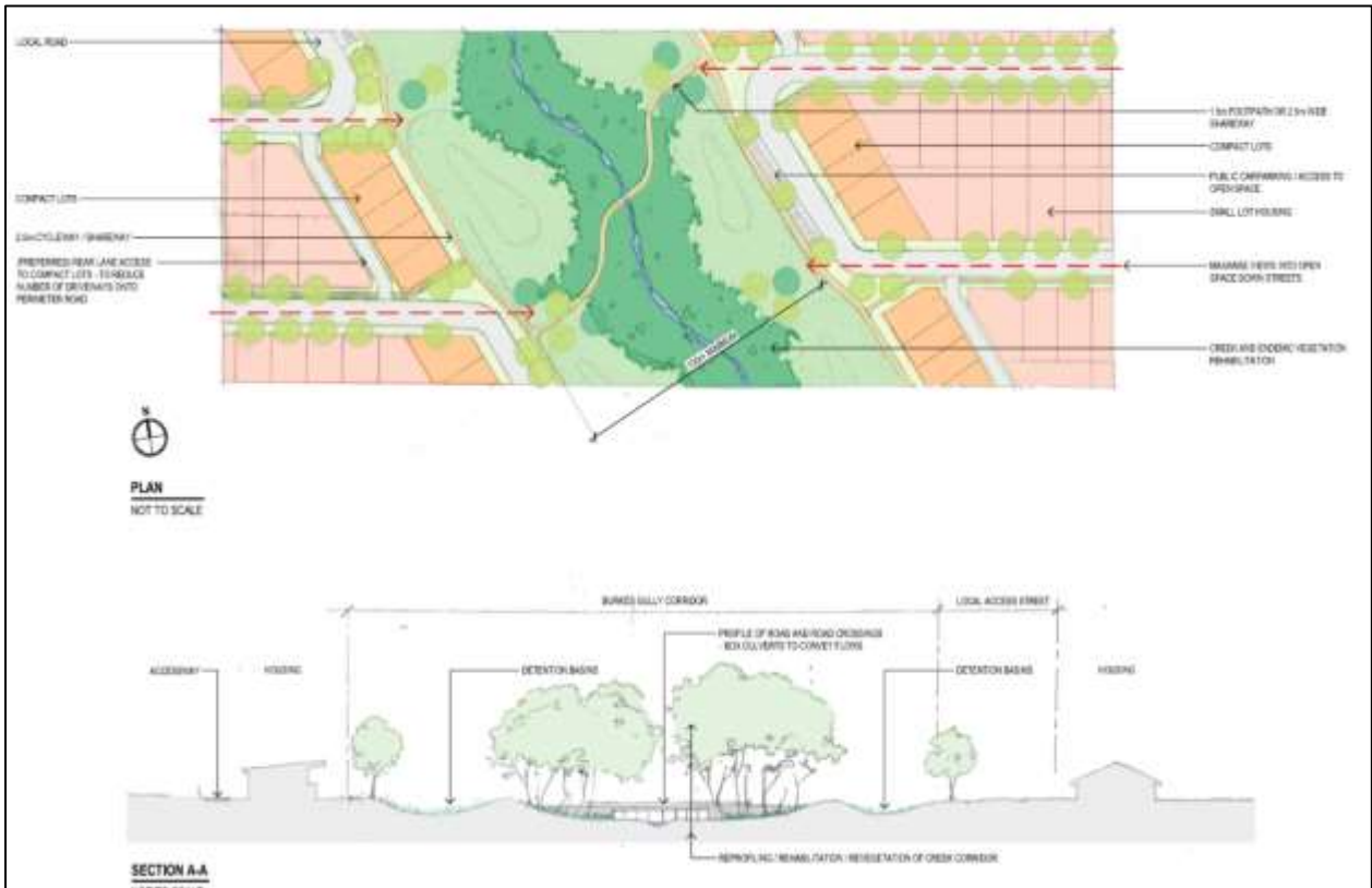
Figure 15: Burkes Gully corridor and section
