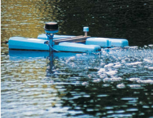
Figure 8. An aerator will help keep algae levels low.
