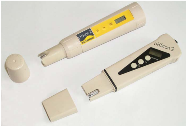
Figure 6. Hand-held pH meters like these are simple to use.
